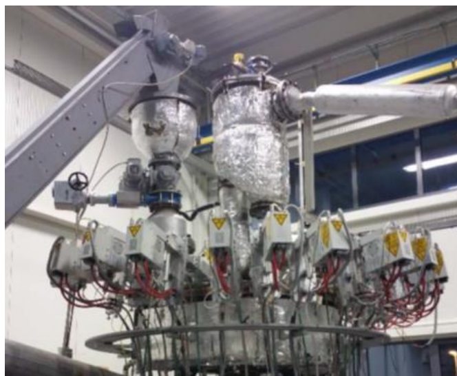
Figure 2: Microwave pyrolysis reactor for Power-to-Liquid applications (installed at Bionic Laboratories BLG GmbH, Germany, www.bionic-world.eu ).
